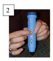
Put the pen into recording state by holding down the mode button for 2-3 seconds - the red light will come on
