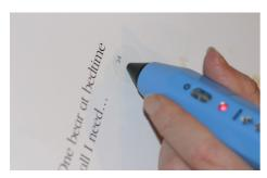
Recordings are saved onto the RecorderPEN's internal hard disk. Each recording is linked to one of the numbered labels. In order to playback recordings the pen must be in 'red' recording mode.
