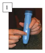
Turn on the pen by holding down the start button for 2-3 seconds the blue light will come on
